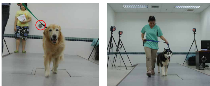
Picture 2. PVF was measured by force plate gait analysis. The velocity of each dog was detected from a reflective target that was attached to each dog's collar (red circle).
